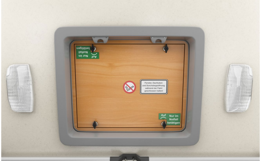
Fig. 3 Access opening in the driver's cab: can be opened downwards in an emergency
